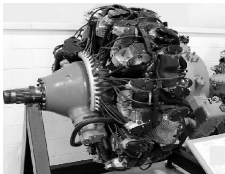
Wright R-3350 18-cylinder radial engine
